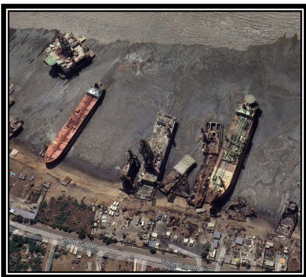
Typical aerial view of Alang from Google Earth in 2022, © 2024 Airbus, showing offshore assets: a semi sub, a drill ship, possibly a barge conversion and an FPSO with turret.
