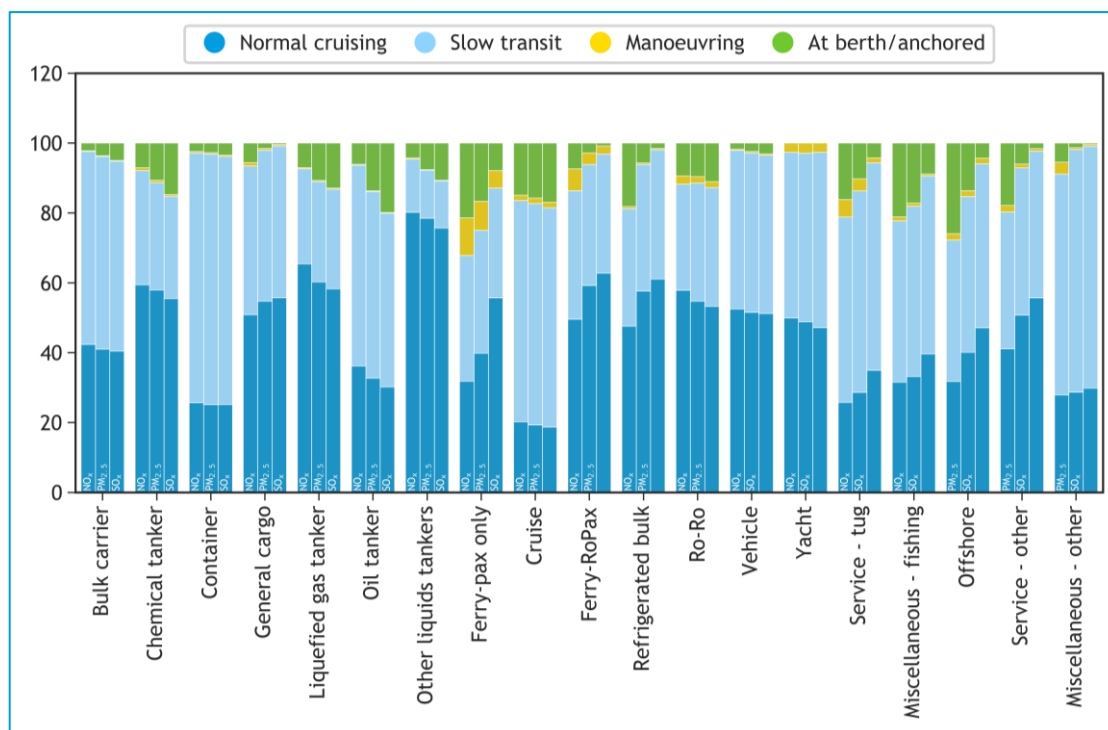
Figure 79 - Proportion of species-specific emissions (NO x , PM 2.5 and SO x ) by operational phase in 2018, according to voyage-specific assignment of emissions. Operational phases are assigned based on the vessel's speed over ground, distance from coast/port and main engine load (see Table 16).
