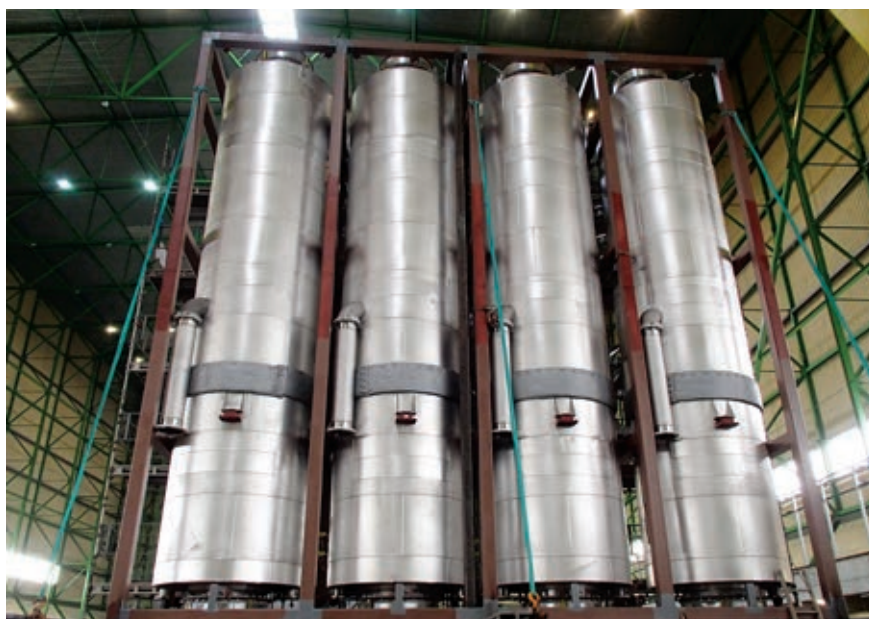
Reducing marine sulphur emissions. A modern scrubber system. (Photo: Wärtsilä Corporation)
